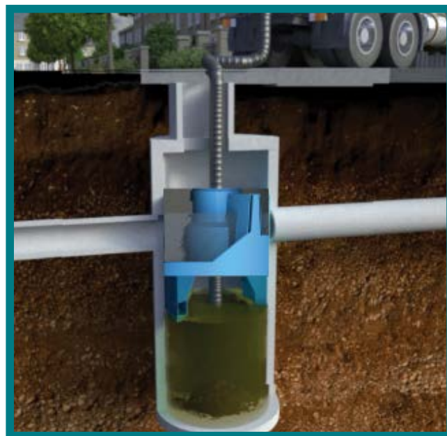
Fig 3. Maintenance is done with a vector truck
